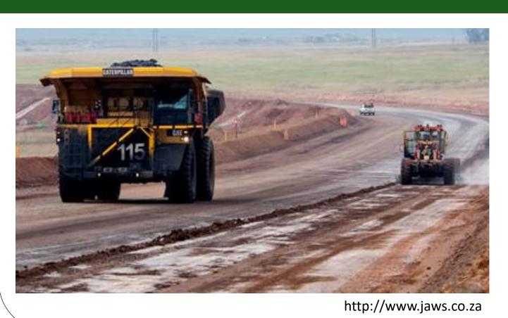
The GPS and vibration data of two haul trucks from a metal mine are collected for a 1-week time frame. The GPS unit natively produces the location, speed, heading, and slope. The mine is subdivided into small road sections, approximately the size a road maintenance crew would service. In total, over 400,000 observations were collected. [2]
